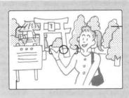
When the shutter release button is depressed half way, the focus and exposure settings are locked on that part of the subject centered within the focusing frame (Focus lock / AE lock function).
